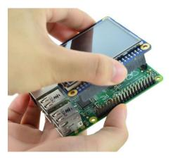
**NOTE:** The 4DPi-24-HAT is supported only by the 40 way header, and therefore pressing on the touch screen may result in the 4DPi-24-HAT moving towards the Raspberry Pi, and therefore the circuitry touching the Raspberry Pi. This could result in damage to either product if a short circuit were to occur. It is therefore highly encouraged to mount the display on the Pi using standoffs (not supplied). Some options are available from places like Mouser.
