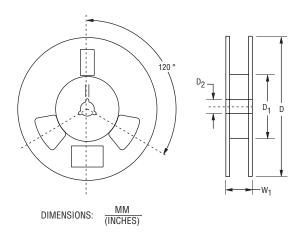
Devices are packed in accordance with EIA standard EIA-481-D and specifications shown here.
