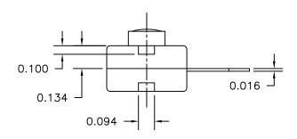
JUDCO INVENTORY NO. 50-0014-00 SWITCH TYPE: PUSH BUTTON, SPST, ON-OFF ELECTRICAL RATING: 12 VDC, 500mA
