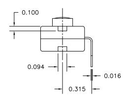
JUDCO INVENTORY NO. 50-0015-00 SWITCH TYPE: PUSH BUTTON, SPST, ON-OFF ELECTRICAL RATING: 12 VDC, 500mA
