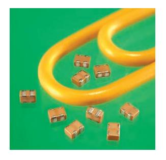
Capacitor arrays combine separate multi-layer ceramic capacitors of the same value in a single passive component. The primary advantages of this device are a reduction in PCB space and placement time. The arrays are offered in three standard dielectrics and feature barrier terminations and tape & reel packaging.
