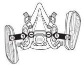
Turn adapter <sup>1</sup>/<sub>4</sub> turn clockwise to stop. To remove adapter, turn <sup>1</sup>/<sub>4</sub> turn counterclockwise.
