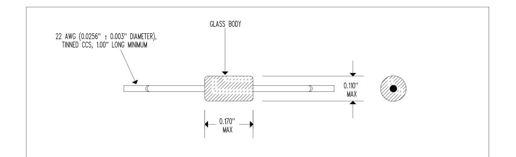
RESISTANCE @  $+25^{\circ}C = 5,000 \ \Omega \pm 10^{\circ}$ RESISTANCE/TEMPERATURE CURVE = "J"
