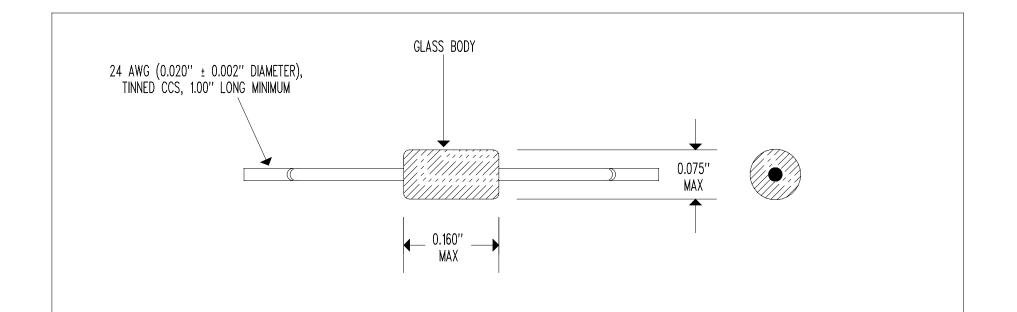
RESISTANCE @  $+25^{\circ}C = 50,000 \ \Omega$  NOMINAL ACCURACY (0 TO  $+100^{\circ}C) = \pm 0.50^{\circ}C$  RESISTANCE/TEMPERATURE CURVE = "J" TEMPERATURE COEFFICIENT @  $+25^{\circ}C = -4.4\%$ /C NOMINAL BETA " $\beta$ " (0 TO  $+50^{\circ}C) = 3,892^{\circ}K$  NOMINAL DISSIPATION CONSTANT = 2 mW/°C NOMINAL (STILL AIR) THERMAL TIME CONSTANT = 5 SECONDS NOMINAL (STILL AIR) THERMAL TIME CONSTANT = 0.5 SECONDS NOMINAL (WELL STIRRED OIL) MAXIMUM TEMPERATURE RATING =  $+300^{\circ}C$
