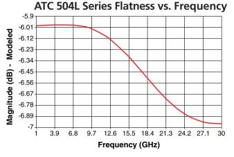
Modeled with HFSS using Rogers 3003 substrate, with a thickness of 10 mils and a line width of 24 mils, representing data for 100 Ohms.
