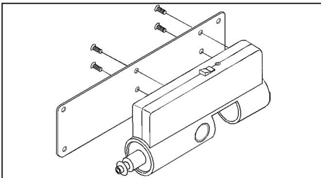
*Figure 5: Mounting the console to the mounting plate*
