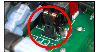
Figure 6. 220V jumper setting
