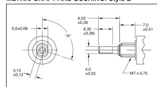
Metric standard dimensions for the shaft and bushing are shown in the drawing. Other dimensions approximately the same as shown in dimensional drawing. Contact Grayhill for exact dimensions. See Style "E" in the Choices and Limitations chart.
