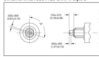
Form, fit and function equivalent to standard shaft switches. The dimensions shown have evolved as the most popular for this type of switch. See Style "B" in the Choices and Limitations chart. Previous users may have ordered these switches by a non-descriptive part number containing a "Y". Contact Grayhill, if in doubt about a cross-reference.
