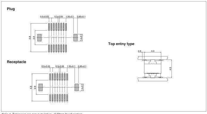
Note: 1. Tolerances are non-cumulative: ±0.03mm for all centers. 2. The dimensions above should serve as a guideline. Contact JST for details.
