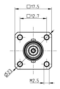
All dimensions are in mm; tolerances according to ISO 2768 m-H
