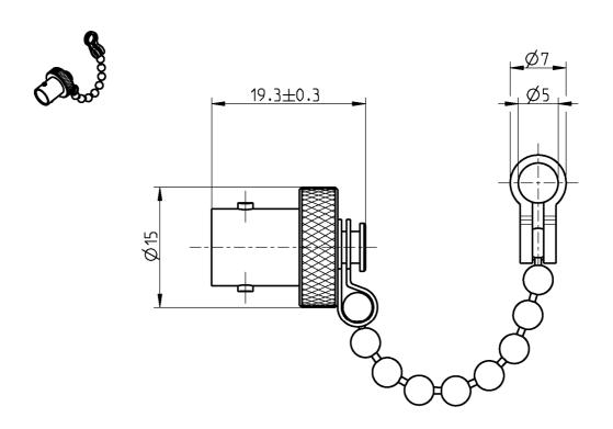
chain of balls stretched length with loop 86mm
