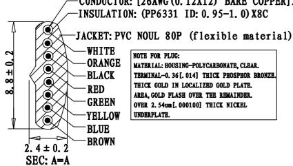
NOTE FOR PLUG: MATERIAL: HOUSING-POLYCARBONATE, CLEAR. TERMINAL-0. 36[. 014] THICK PHOSPHOR BRONZE. THICK GOLD IN LOCALIZED GOLD PLATE. AREA, GOLD FLASH OVER THE REMAINDER. OVER 2.54um[.000100] THICK NICKEL UNDERPLATE.
