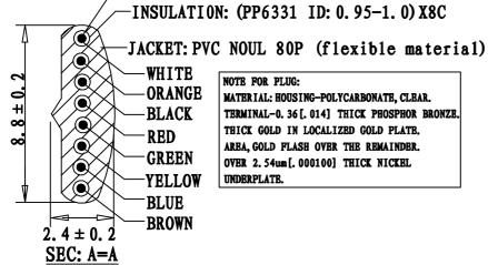
NOTE FOR PLUG: MATERIAL: HOUSING-POLYCARBONATE, CLEAR.
