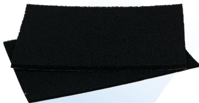
Part Number 5206 is a lightweight lossy foam sheet absorber, which achieves a broad frequency range of dielectric loss through a carbon coating. 5206 has similar performance to PN5103, but has no sulfur in its formulation. Surfactants used in industry carbon latex coatings have small amounts of sulfur in them. This can cause corrosion inside of electronic housings in certain application. PN 5206 has no sulfur in the coating and eliminates this problem.
