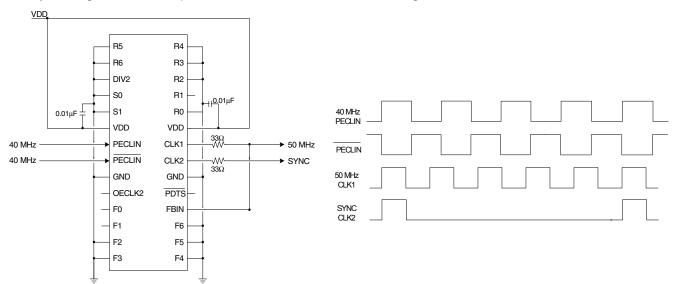
Note: The series termination resistor is located before the feedback trace.
