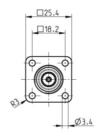
All dimensions are in mm; tolerances according to ISO 2768 m-H
