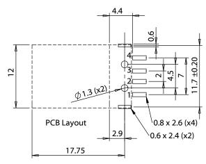
**DIMENSIONS ARE IN** MILLIMETERS
