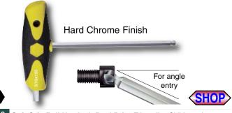
540 Soft Grip Ball Hex Inch Dual Drive T-handle CVM steel, hardened, hard chrome finish. Ball tip for speed & easy insertion. Wiha soft grips are molded on with through the handle side torque drive.
