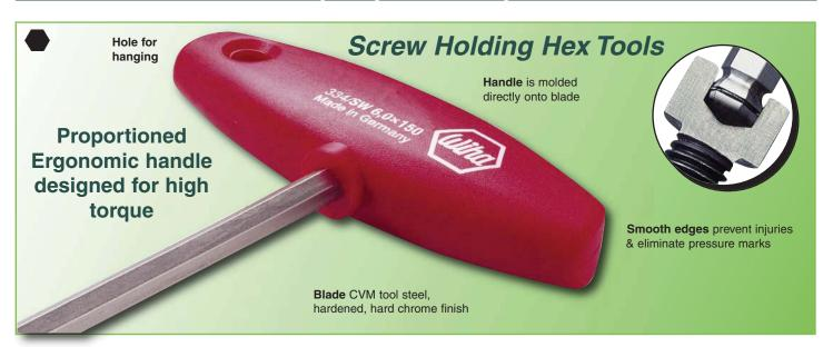
MagicRing Ball End, With Wiha T-handle Blade CVM steel, hardened, hard chromed. Ball end for easy insertion. Wiha T-handle high quality plastic, impact resistant.
