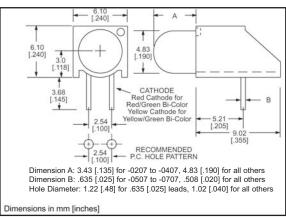
Standard Polarity shown in drawing: Cathode right
