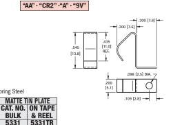
Tape and Reel Spec's: 32mm wide; 16mm pitch; 13 inch reel (250 pieces per reel)
