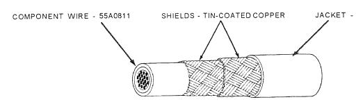
JACKET - RADIATION-CROSSLINKED, MODIFIED ETFE
