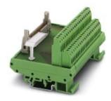
VARIOFACE module, with screw connection and flat-ribbon cable connector, for mounting on NS 32 or NS 35/7.5, with pin strip and short and long locking latches for socket strips, 16-pos.
