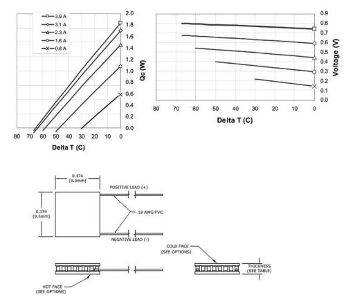
Ceramic Material: Alumina (Al<sub>2</sub>O<sub>3</sub>) Solder Construction: 138°C, Bismuth Tin (BiSn)
