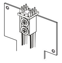
**Step 1:** Mount the HM55B Compass Module on the back side of the PING))) Mounting Bracket using (2) 4/40 ½" screws, (2) 4/40 nuts and (2) 10" servo extension cables.
