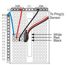
The PING))) sensor requires a 5 VDC power supply. To make the connections directly from the breadboard:
