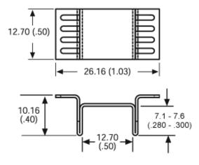
Note: The thickness of the drain pad is variable depending on the amount of heat generated by the SMT device, design, limitations and process. This is the exposed printed circuit.
