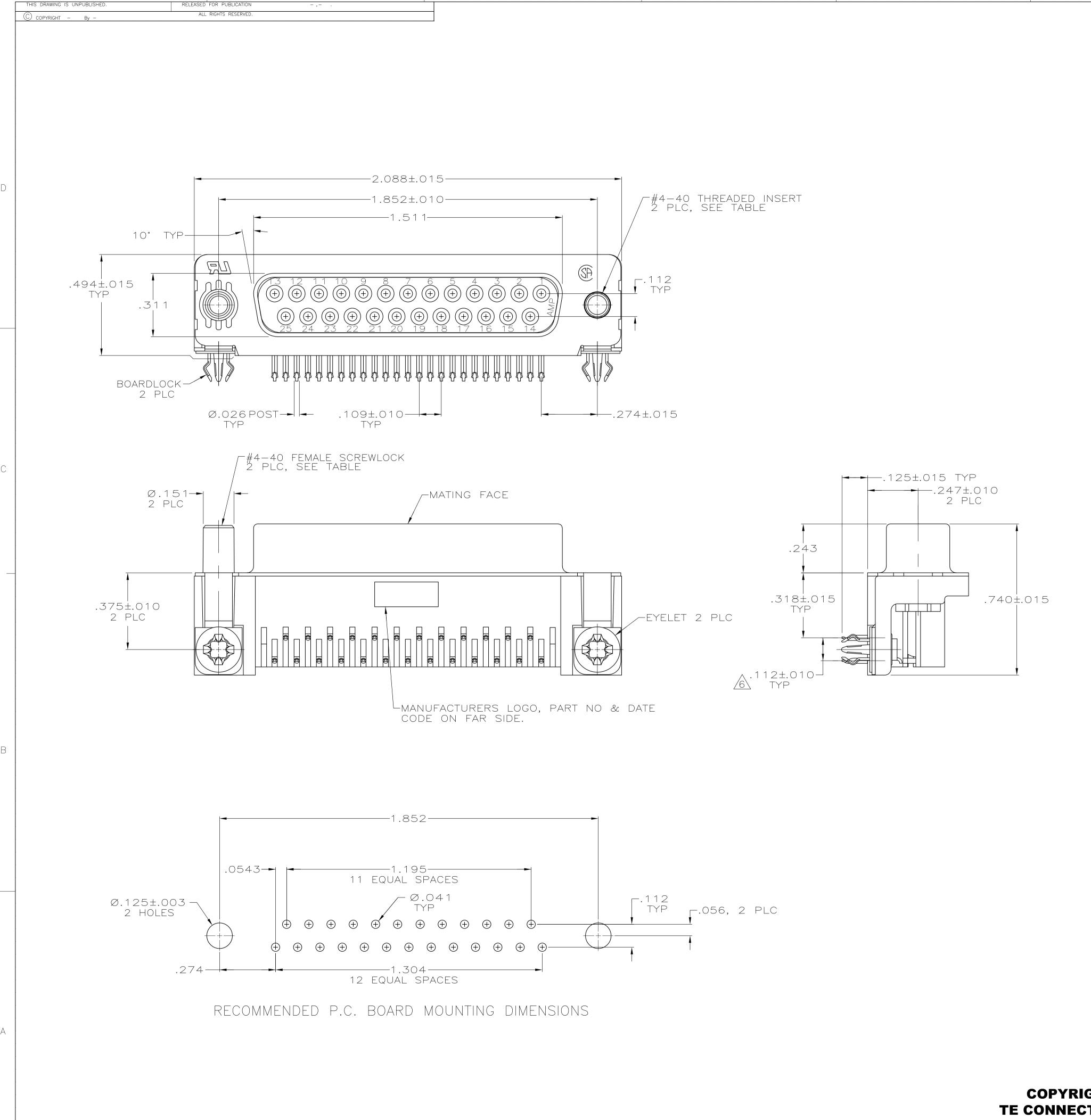
1. CONNECTOR MATES WITH ANY 25 POSN PLUG IN AMPLIMITE SERIES.
