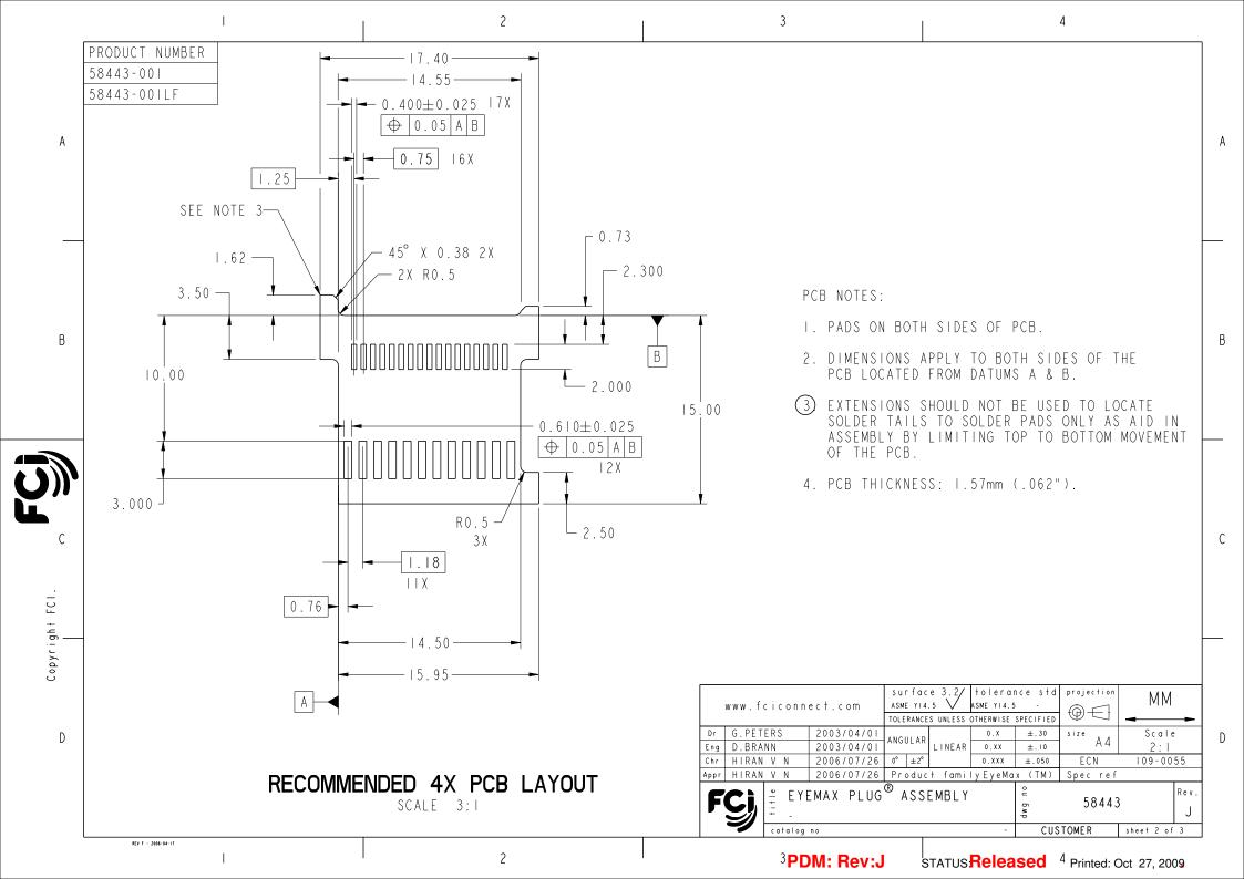
I. MATERIAL: HOUSING, HIGH TEMPERATURE THERMOPLASTIC, UL 94V-0 RATED, SUITABLE FOR REFLOW SOLDERING. CONTACTS: COPPER ALLOY.
