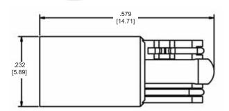
Measurements are typical Dimensions are inches [mm]
