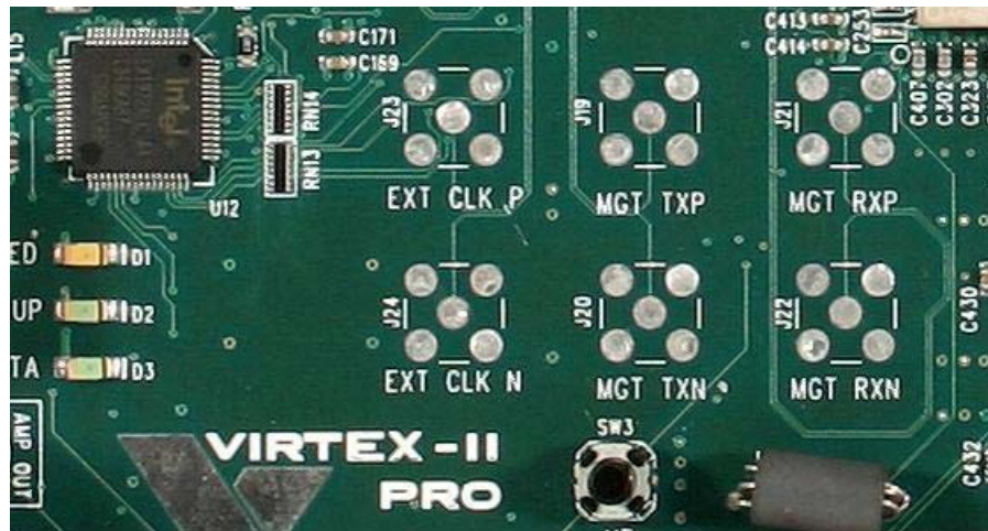
Figure 2-4: External Differential Clock Inputs
