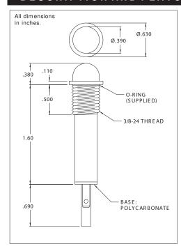
Solid-state indicator lights complete with built-in current-limiting resistor and rectifier diode.
