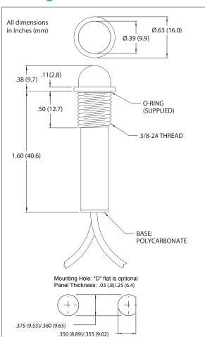
Solid-state indicator lights complete with built-in current-limiting resistor and rectifier diode.
