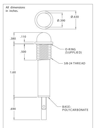
Solid-state indicator lights complete with built-in current-limiting resistor and rectifier diode.
