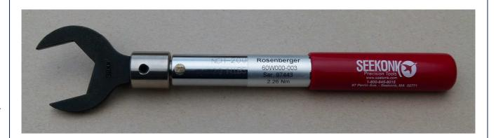
This Torque Wrench is specially set to a low torque that makes it useable for metrology purposes like direct connections on vector network analyzers (VNA) and calibration kits. The high torque that is normally used for 7-16 connectors can destroy the VNA test port and leads to high abrasion on test port connectors and calibration standards. This Torque Wrench should not be used for durable outdoor connections, high power or low PIM applications!
