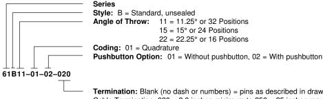
**Termination:** Blank (no dash or numbers) = pins as described in drawing Cable Termination 020 = 2.0 inches minimum to 250 = 25 inches maximum. Provided in increments of 1/2 inch. Example 035 = 3.5", 060 = 6 inches. Cable is terminated with standard Amp Connector 640442-6. Use any 6 position, .100 center header to mate with the cable assembly. Contact Gravhill
