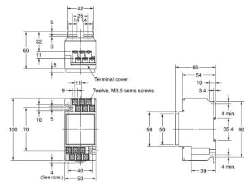
Note: Dimensions are with the DIN rail mounting (sliding) bracket attached.
