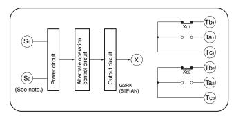
$\left( \begin{array}{c} \textbf{Note:} \text{ The above diagram is for a rated voltage of 200 or 220 VAC.} \\ \textbf{Power is supplied to $S_0$ and $S_1$ for 100 or 110 VAC.} \\ \textbf{Connections (Refer to connection diagram.)} \end{array} \right)$
