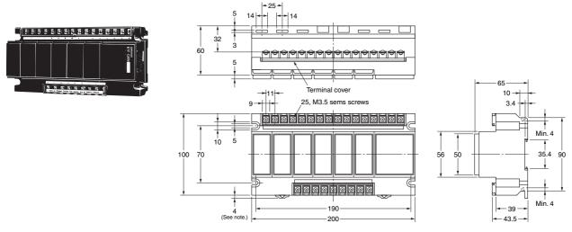
Note: Dimensions are with the DIN rail mounting (sliding) bracket attached.
