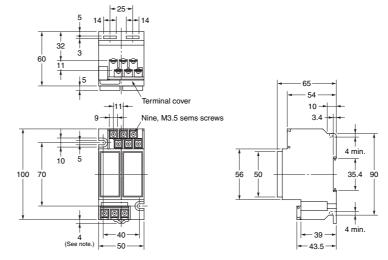
Note: Dimensions are with the DIN rail mounting (sliding) bracket attached.
