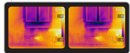
Original IR Image on the Left and with MSX ™ Enhancement on the Right image
