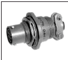
62 IN - 14F Single hole mounting with grommet and grommet nut fitted with integral strain relief clamp has panel 'O' ring seal
