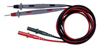
Model **6264**: Body – Steel, Nickel Plated, Insulation – Polypropylene fire retardant, Spring: Music Wire, **RATINGS**: IEC 61010-031, Category III, Operating Voltage: 300 V, Current: 3 Amperes.
