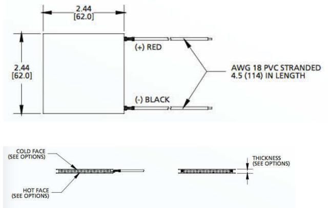
Ceramic Material: Alumina (Al<sub>2</sub>O<sub>3</sub>) Solder Construction: 138°C, Bismuth Tin (BiSn)
