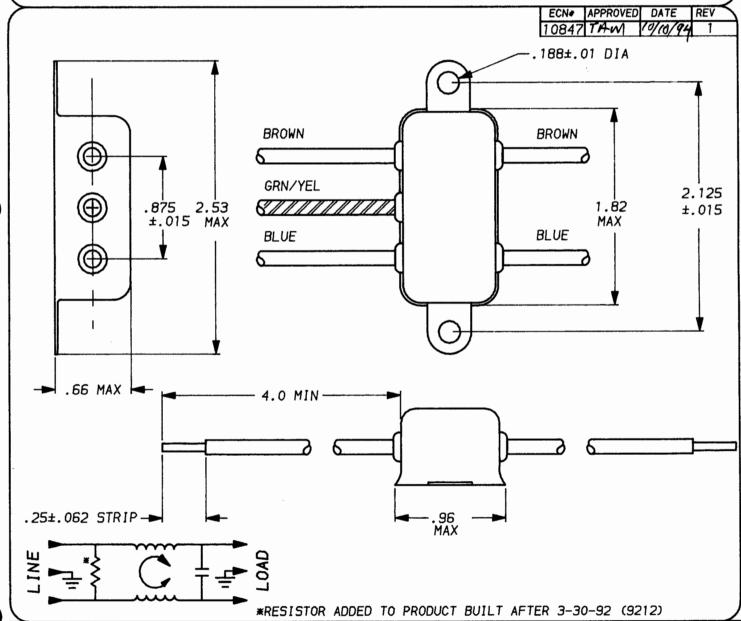
UNLESS OTHERWISE SPECIFIED, 50p - 50p (MINIMUM) INSERTION LOSS TOLERANCE TO BE ±.025 FREQUENCY .15 .50 1.0 5.0 10 20 MHz MATERIAL & FINISH: AS SUPPLIED POWER LINE FILTER COMMON This document is proprietary to CORCOM INC. and is not to be reproduced nor used for manufacturing purposes except on CORCOM'S prior written consent. 13 15 17 16 15 14 dB DATE: 10-4-94 DIFF. APPRVD. 1 0EH3 01 dB
