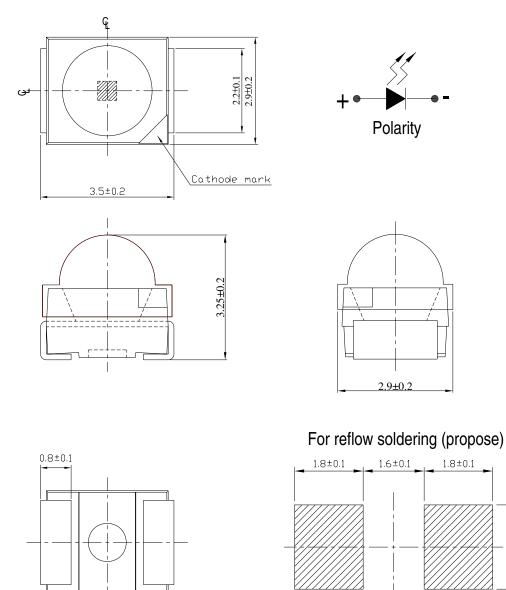
**Notes:** 1.All dimensions are in millimeters 2.Tolerances Unless Dimension = ±0.1mm
