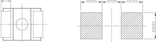
**Notes:** The tolerances unless mentioned is  $\pm 0.1$ mm, all dimensions are in millimeters.
