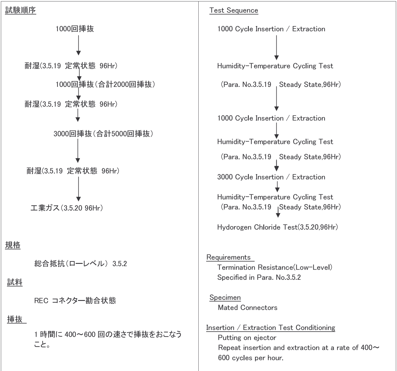
Fig.3 挿抜耐久性(オフィス外環境 5000 回) Fig.3 Durability Test (Harsh Environment)
