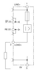
operating condition: SF +24 V = OK fault condition: SF 0 V
