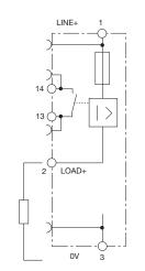
operating condition: 13-14 closed fault condition: 13-14 open
