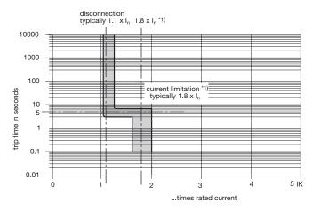
$<sup>^{*1)}</sup>$  current limitation typically 1.8 x I<sub>n</sub> times rated current at I<sub>n</sub> = 0.5 A...6 A current limitation typically 1.5 x I<sub>n</sub> times rated current at I<sub>n</sub> = 8 A or 10 A current limitation typically 1.3 x I<sub>n</sub> times rated current at I<sub>n</sub> = 12 A
